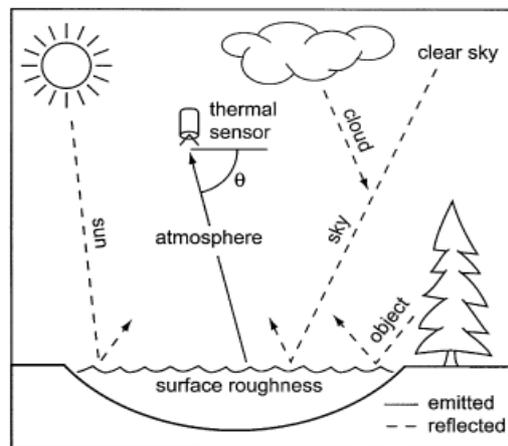
Fig.1. Sources of emitted and reflected radiation in thermal remote sensing of rivers
