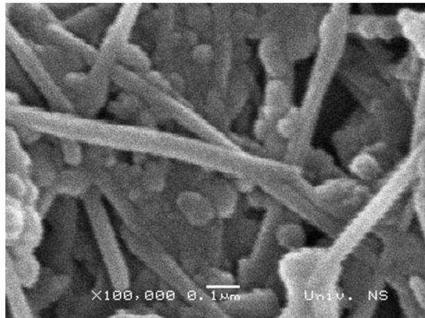
**Figure 3. MWNT after PmPV purification.
