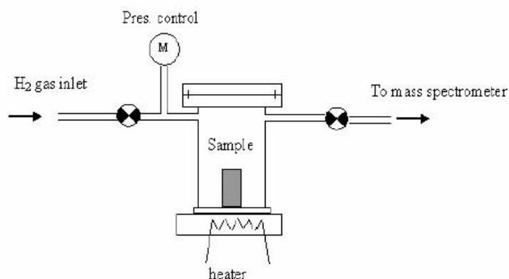
**Figure 1. Schematic diagram of chamber for adsorption hydrogen**
